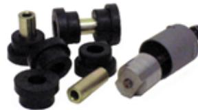
A safety test weakspot on the Jaguar XJ and XJS models has always been the steering rack mounting bushes. When these deteriorate it leads to vague steering and unpredictable handling.
