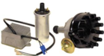
The Opus ignition system as fitted to V12 models is notoriously unreliable! Despite being relocated to the front of the engine on later models, away from the heat in the Vee, they are still extremely troublesome. Sometimes the problem is hard to pinpoint as it is often intermittent before the unit fails altogether. Depending where you are at the time that can be anything from inconvenient to plain embarrassing!
